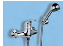
Art. 048/E MISCELATORE MONOCOMANDO DOCCIA ESTERNO Duplex con flessibile mm. 1500, eccentrici da 1/2 " regolabili per interasse da mm. 150 ± 15 EXTERNAL SINGLE LEVER SHOWER MIXER Duplex with shower hose mm. 1500, s-tailpieces with 1/2" connections, centre distance mm 150 ± 15
